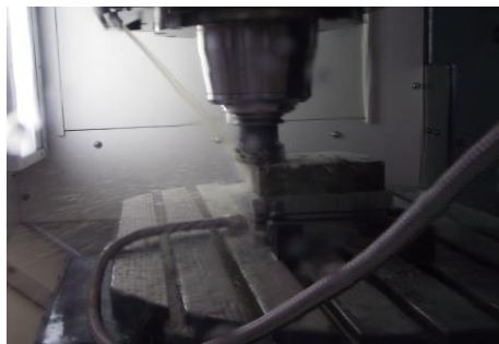
Asymmetrical cut-down milling with \Psi < 90^\circ
